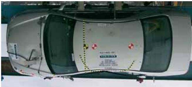
Figure 3 - 302mm deformation of a 2002 Toyota Camry as a result of a 62km/h side impact moving barrier (broad object at least 1500mm wide) test
