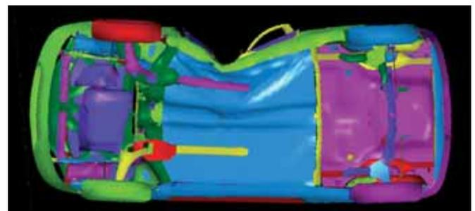
Figure 10 - 20km/h lateral pole impact (bottom view)
