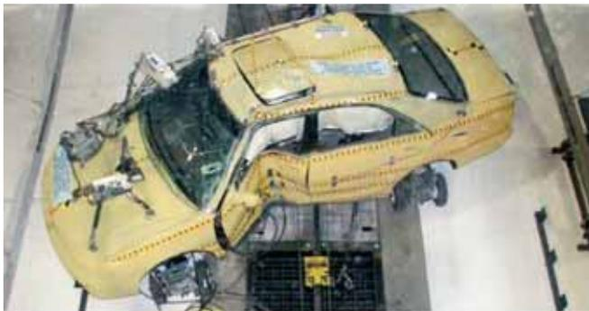
Figure 2 - 412mm deformation of a 2003 Toyota Camry as a result of a 32km/h lateral pole impact (254mm) test
