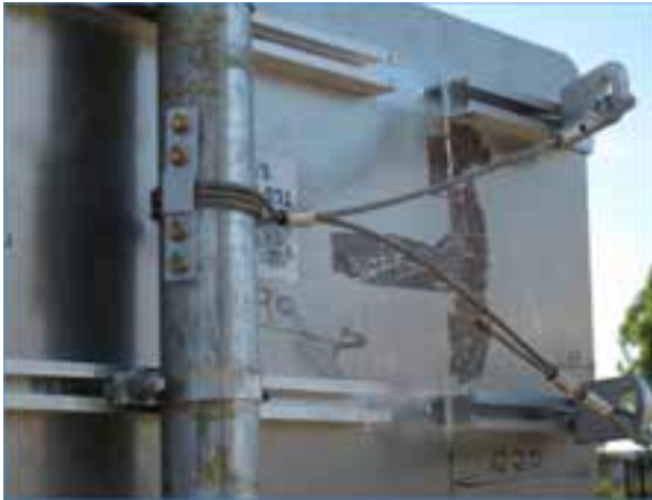
Figure 5. Test 3 – left - cut rails & stainless rope tether, right- successful crash deflection crash
