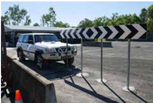
Figure 2. Test 1 – sign layout & vehicle damage after crash
