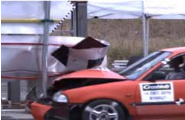
Figure 11. Test 7 – left-small vehicle on impact, right- large area signs & large posts
