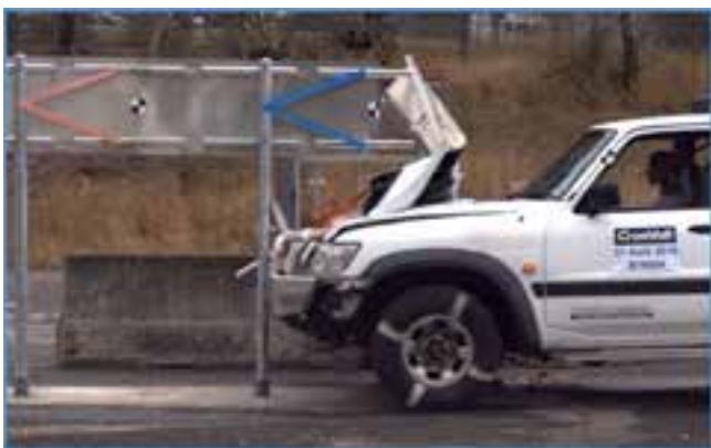
Figure 6. Test 4 - cut rails & flat straps
