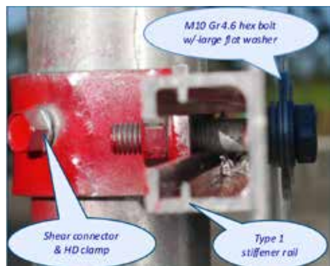
Figure 7. Test 5 onward – heavy duty clamps used
