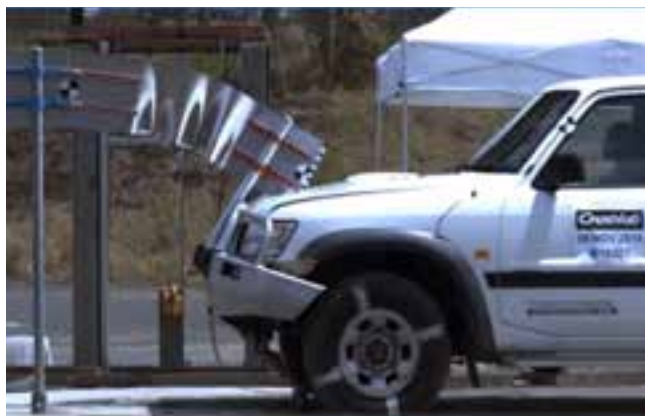
Figure 8. Test 5 - Shortened rails & HD anchored clamps
