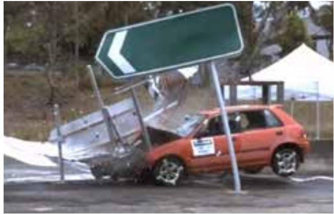
Figure 11. Test 7 – left-small vehicle on impact, right- large area signs & large posts
