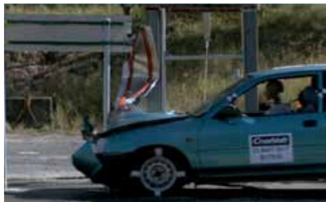
Figure 15. Test 10 – successful use of HD clamps & bolted through design
