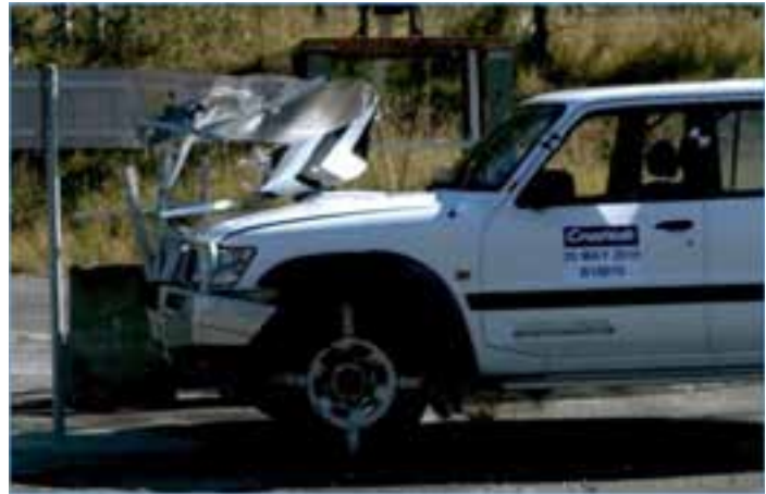
Figure 5. Test 3 – left - cut rails & stainless rope tether, right- successful crash deflection crash
