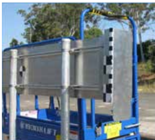
Figure 3. Test 2 - sign end reinforcement
