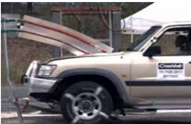
Figure 12. Test 8 – No through bolts and slicing of the bonnet
