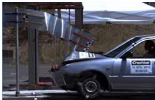
Figure 9. Test 6 - Shortened rails & HD anchored clamps
