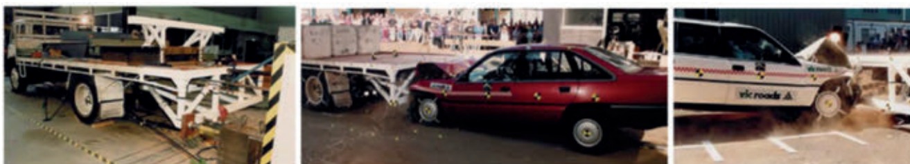
Figure 3. RUPD rigid barrier design (Rechnitzer, Powell &amp; Sayer, 2001)
