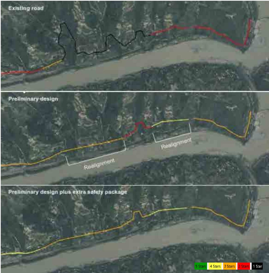
Figure 4. Targeted improvements to designs in Shaanxi, China
