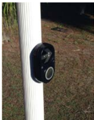
Figure 7. Bicycle activated warning sign push button
