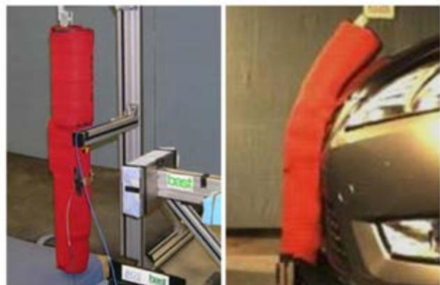
Figure 2. The Flex-PLI is used from 2014 to assess pedestrian knee and tibia injury risk.
