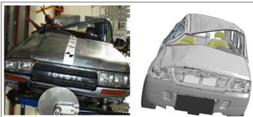
Figure 4. Vehicle permanent deformation - comparison between experimental test (left) and simulation (right)
