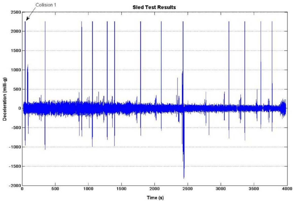
Figure 6: X-deceleration against time for the entire testing period of the sled test
