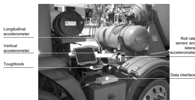
Figure 1. Instrumentation fitted to test vehicle
