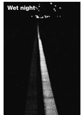
Only the "Visibead" painted pavement marking is visible when it starts to rain.
