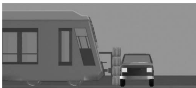
Figure 2: Illustration of improved collision interface compatibility at a level crossing between a vehicle and train with front airbag deployed
