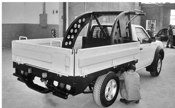
Figure 8: (Above and Below left) The "SWAN" ROPS fitted to utility type vehicles to provide occupant compartment protection a rollover
