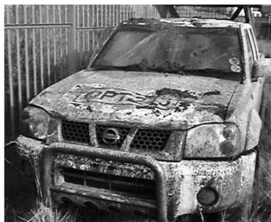
Figure 9: (Above Middle & Bottom) Third rollover of a vehicle equipped with Swan ROPS resulting in maintenance of occupant survival space and only minor injuries.
