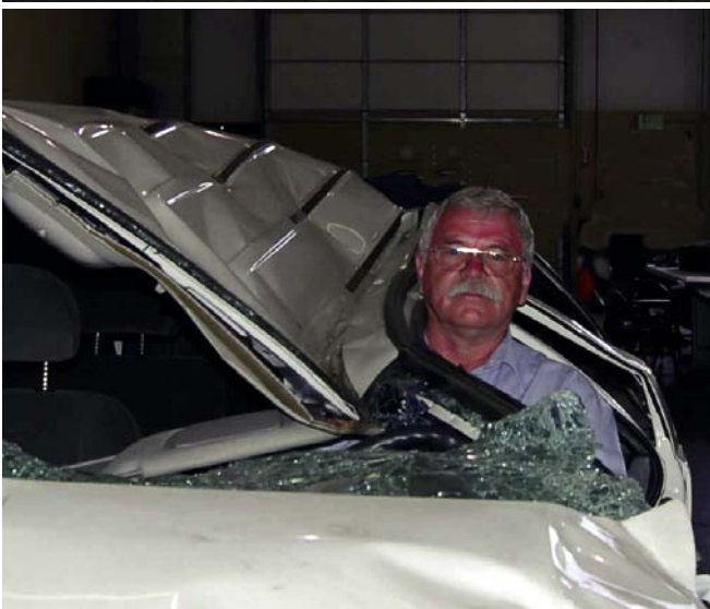
Figure 1: Tenting roof crush and pillar deformation leaves little room for survival
