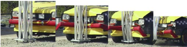
Obligatory EN 12767 low speed 4425 NE test (35 km/h = 21.0 miles/h).
