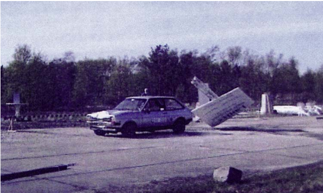
Sign and mast falling close to its original position after impact
