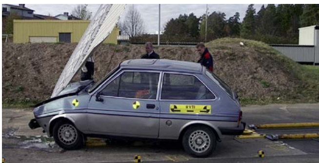
Picture shows a LE Sign Post trial in Sweden where the Sign wants to go above the car while the mast underneath..... Note This is not a standard Lattix mast, but one we attached permanently to the foundation so it does break free on impact
