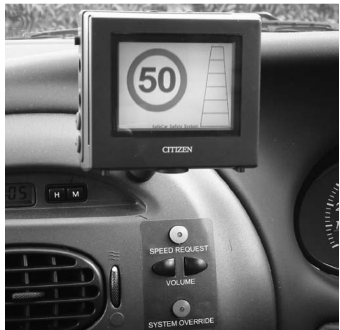
Externally, the test cars looked like other Ford Falcons. The difference was in the dashboard presentation, as shown in this photo.
