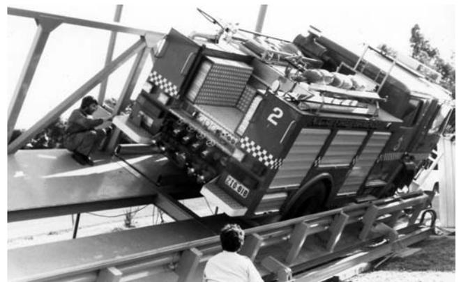
Figure 2. The tilt deck in action – strong chains and stronger nerves required!
