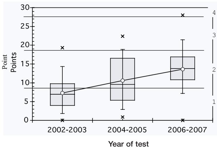
Figure 1 - Box and whisker plot of current Euro NCAP/ANCAP pedestrian test results by test year. ("o" indicates the mean, the box covers the interquartile range, the error bars show 10th and 90th percentile values and "x" shows the highest and lowest values.)
