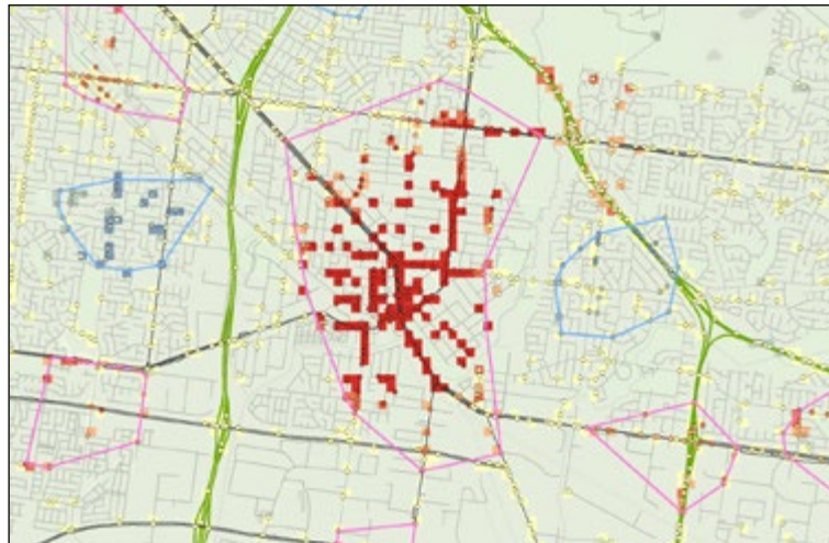
Figure 9. Comparison of aggregation to 100m fishnet (shown as areas) with point aggregation with 10m integration (shown as dots) for identification of hot spots and cold spots for metropolitan Melbourne 2012-2016 casualty crashes – Dandenong zoom
