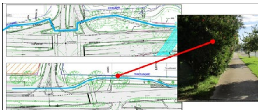
Figure 6. Proposed Design: Shared path with on-road bicycle lane removed (Source: Arcadis Road Design Plan NWA_C1042A and P. Harris)
