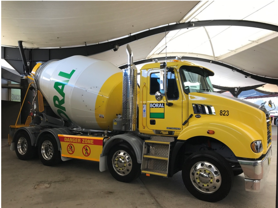
Figure 1. Construction heavy vehicle fitted with blind spot technology and side underrun protection
