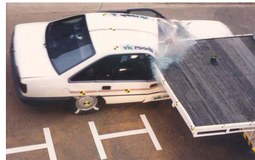
(b) underrun mechanism (after Reznitzner & Grzebieta, 2001)
