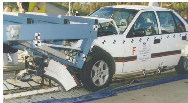
(d) energy dissipating barrier design (after Reznitzner, Powell & Sayer, 2001)
