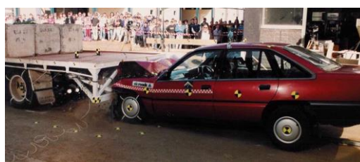
(c) rigid barrier design (after Reznitzner, Powell & Sayer, 2001)
