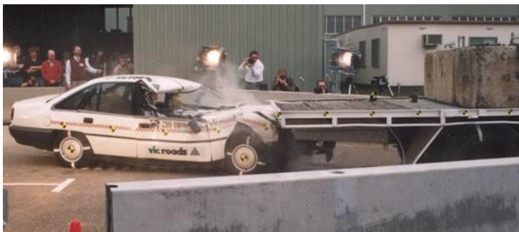
(b) underrun mechanism (after Reznitzner & Grzebieta, 2001)
