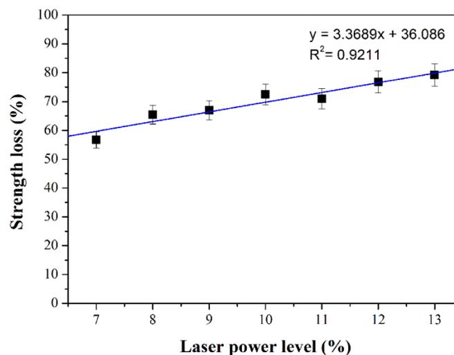
**Figure 2** Relationship between laser power and bursting strength
