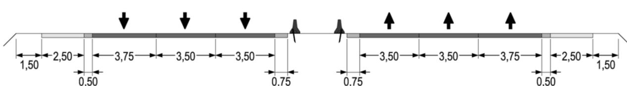
Figure 5. Final position of road safety barriers after road refurbishment
