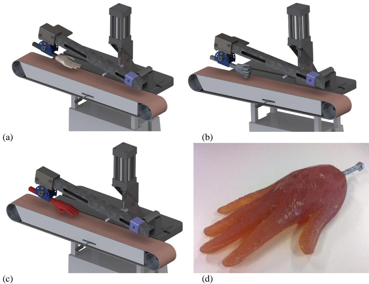
**Figure 1. Concept abrasion tester with hand in the position (a) with outstretched fingers and palm up, (b) the bottom edge of curled fist, (c) outstretched palm of the hand and (d) cast polyurethane hand.**
