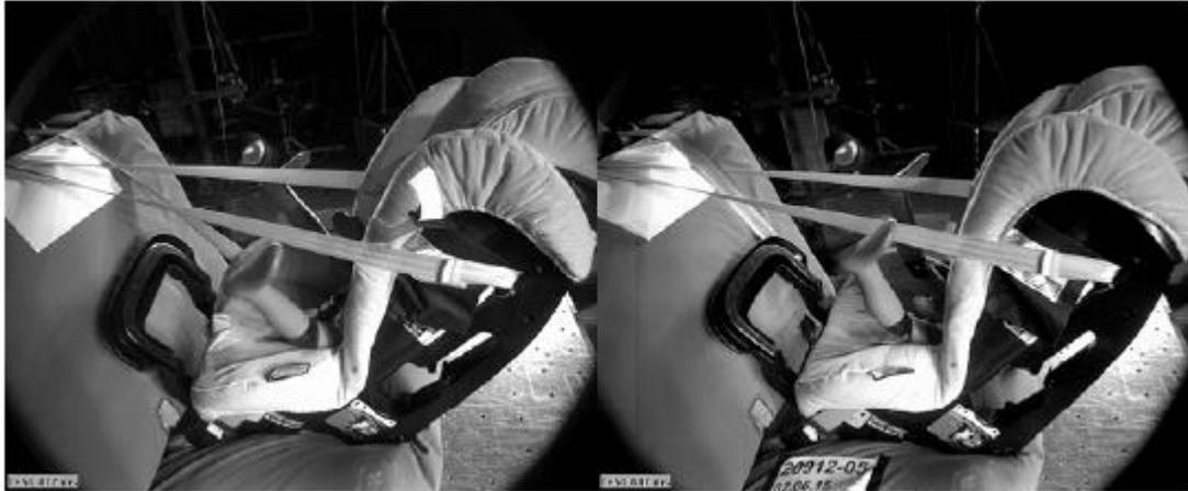
**Figure 4. The restraint twisted less during the gated buckle test (right) when compared to the baseline test (left), at 96ms after impact.**
