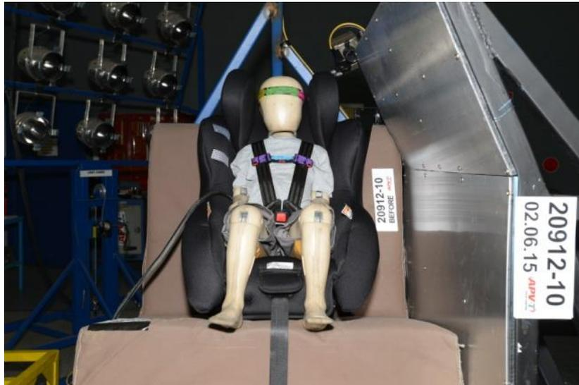
*Figure 8. Chest clip in position before test*
