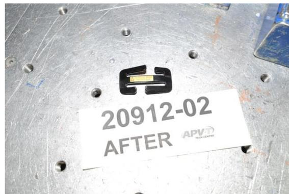
**Figure 7. The bent gated buckle following testing.**
