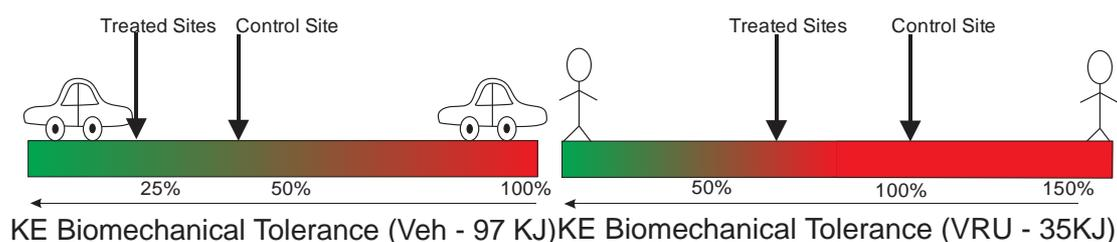
**Figure 1 – relative KE levels for vehicle and vulnerable road user crashes**
