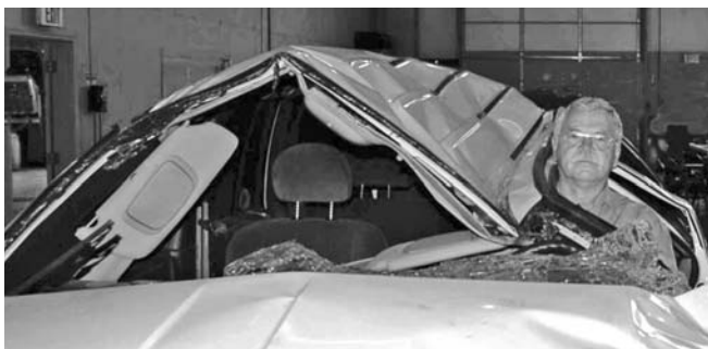
Figure 1: Tenting roof crush and pillar deformation leaves little room for survival
