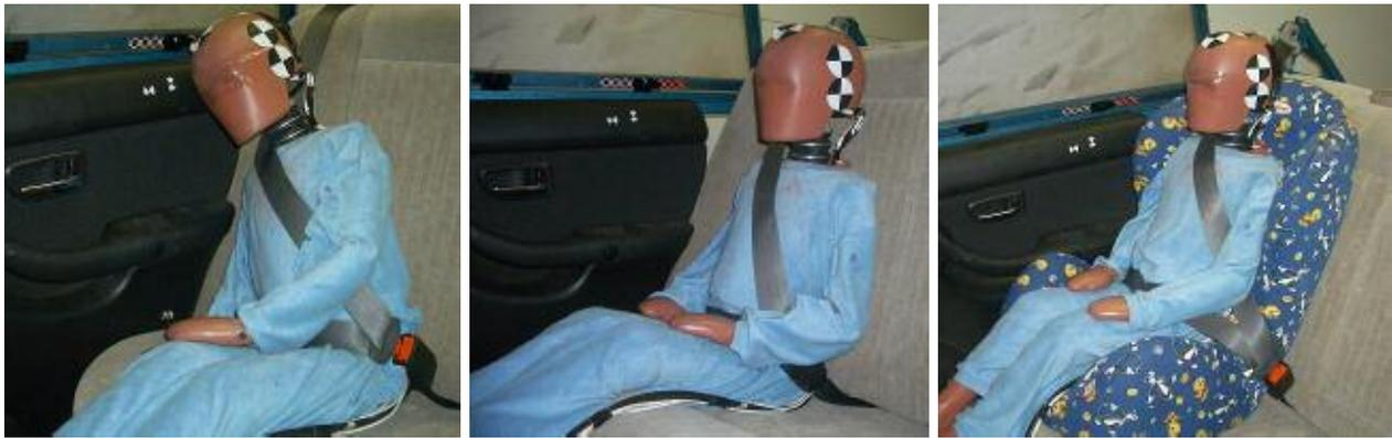
Figure 2. Initial postures for Case 2. Note the position of the sash belt near the neck in the slumped scenario.
