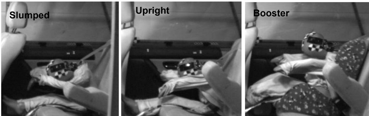
Figure 3. Kinematics of dummy in Case 2. Note the rotation of the dummy in the slumped case compared to the upright and booster scenarios.
