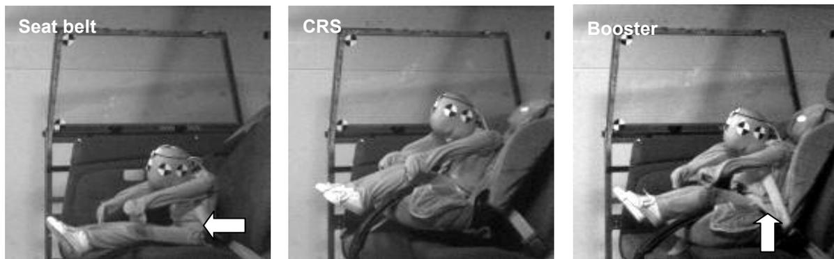
**Figure 1. Position of child dummy at maximum excursion in three different restraint types. Note the position and more horizontal angle of the lap belt in the seat belt condition compared to the booster scenario, where the belt is more angled, and lower on the thighs.**
