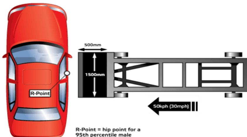
Figure 2 Side Impact Test
