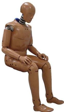
Figure 4 Hybrid III Dummy
