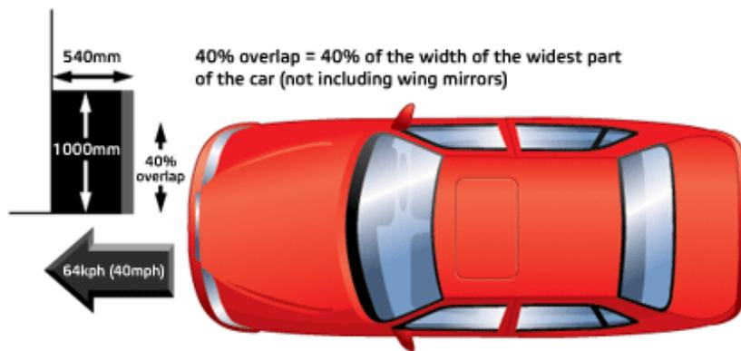
Figure 1 Frontal Offset Test
