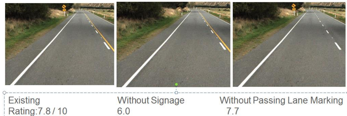
Figure 5. Example of photos showing different Road layouts
