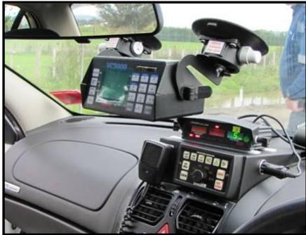
The device is mounted on the test vehicles windscreen and can be activated externally from the brake lights or internally by the deceleration of the test vehicle which in turn is directly related to the braking force.
