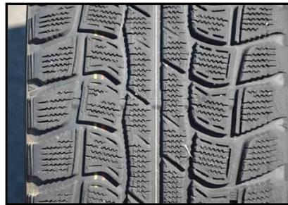
The set of conventional tyres used were from an older style VZ series Holden Commodore Police patrol vehicle. The same conventional tyres were used for all the relevant tests involved in this research.
