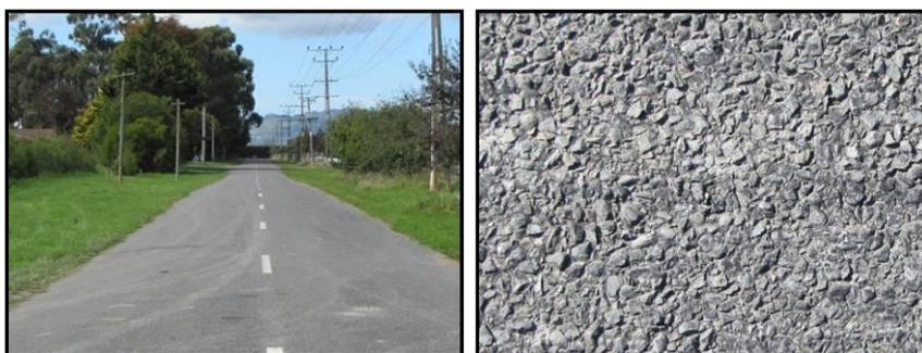
The chip seal is representative of tar sealed chip aggregate used widely in New Zealand. Asphaltic concrete in the full range of mix types is used in more heavily trafficked areas and more common in urban areas where noise is of concern.
