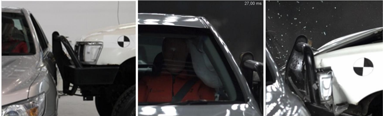
Figure 7. Series of front view of test 5 showing bull-bar rotated backward
