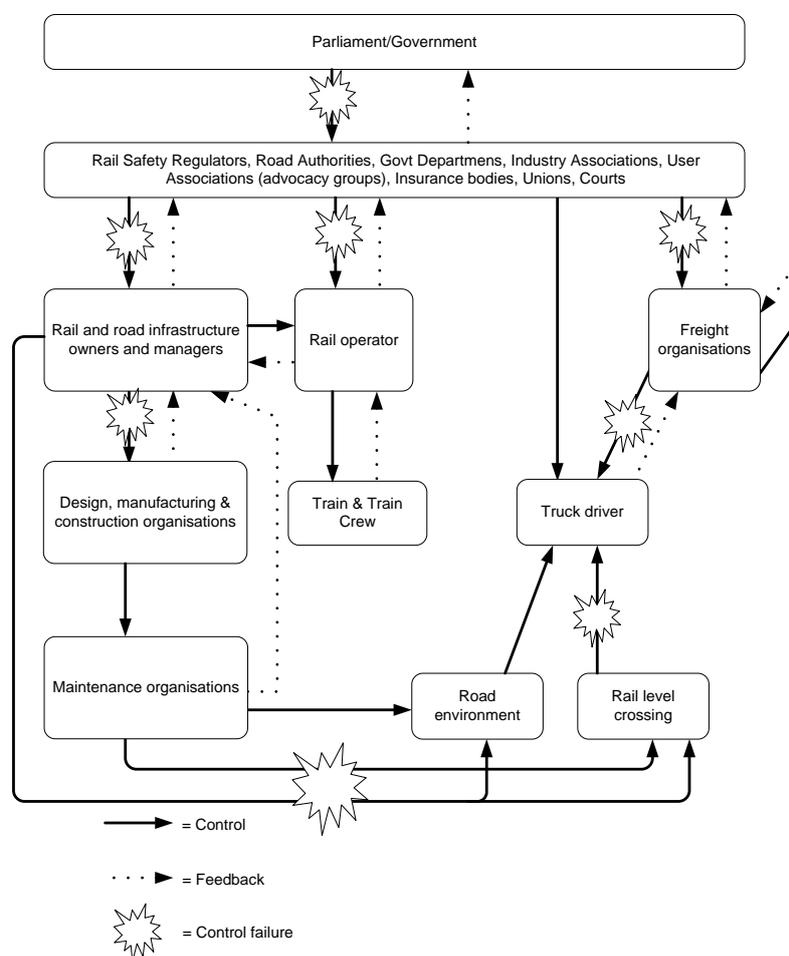
**Figure 3. Rail level crossing control structure with control failures.**
