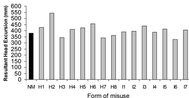
**Figure 2:** Resultant head excursion associated with different forms of FFCRS misuse. The black bar denotes correct use. Definitions of misuse descriptors are given in Table 1.
