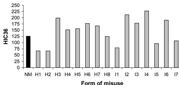
**Figure 1:** HIC values associated with different forms of FFCRS misuse. The black bar denotes correct use. Definitions of misuse descriptors are given in Table 1.
