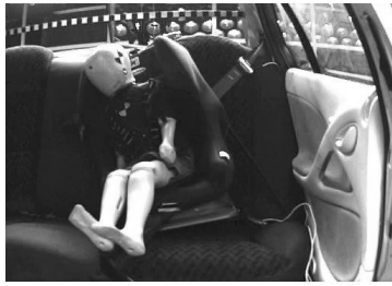
Seatbelt anchorage at impact
