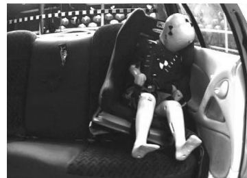
Flexible anchorage in rebound
