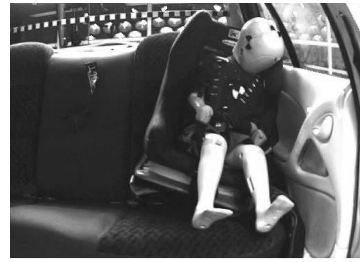
Seatbelt anchorage in rebound
