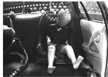
Flexible anchorage in rebound
