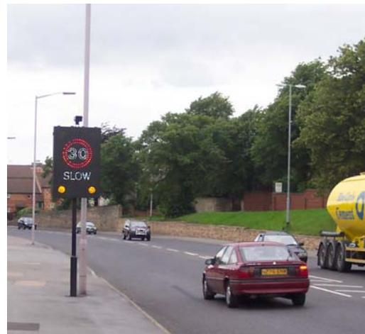
The signs utilise fibre-optic technology or light emitting diodes to display the symbols and/or words required, so allowing different colours to be used for different parts of the message. At night, automatic dimming is used to reduce the intensity of the sign output. Activation of such signs is typically through the use of microwave detectors, although inductive loops cut into the road surface can also be used.
