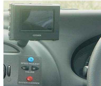
Figure 1. ITS display and control panel
