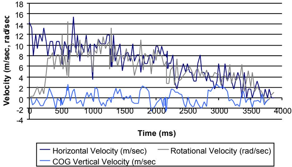
**Figure 2:** Comparison of principal velocities of the vehicle during the Malibu II Test 3 rollover crash test.
