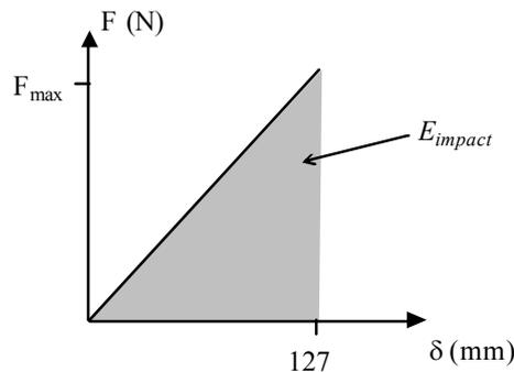
Figure 4: Energy absorbed ( $E_{impact}$ ) by the vehicle's roof deforming elastically
