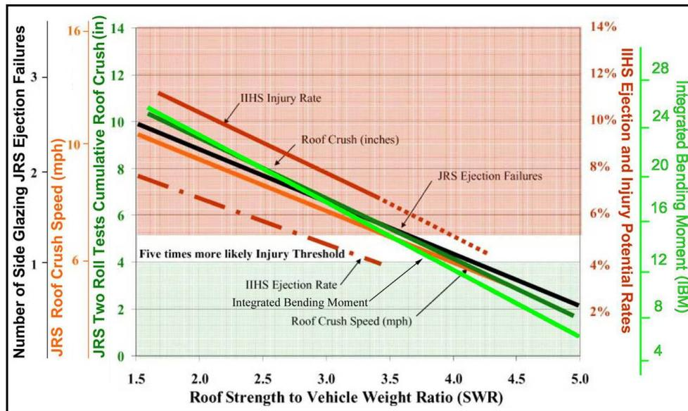
Figure 1: Comparison of IIHS injury rate and JRS injury criteria for different roof strengths [8]
