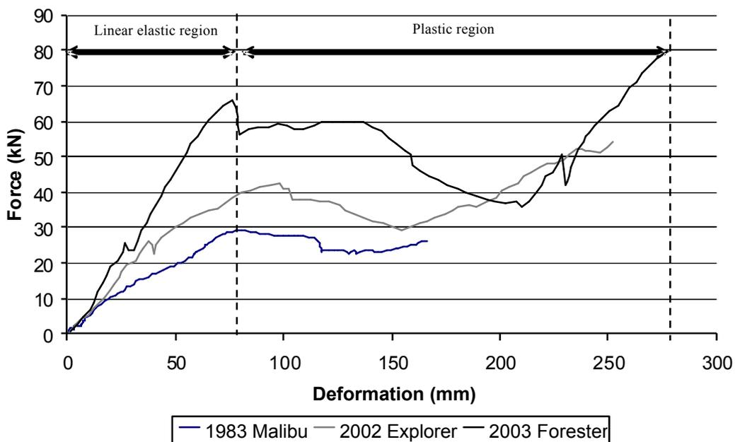
Figure 3: Comparison of FMVSS 216 deformation for a range of vehicles [14, 16]
