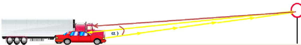
**Diagram 7: Demonstrates differences in observation angle for a driver of a car compared to a truck**
