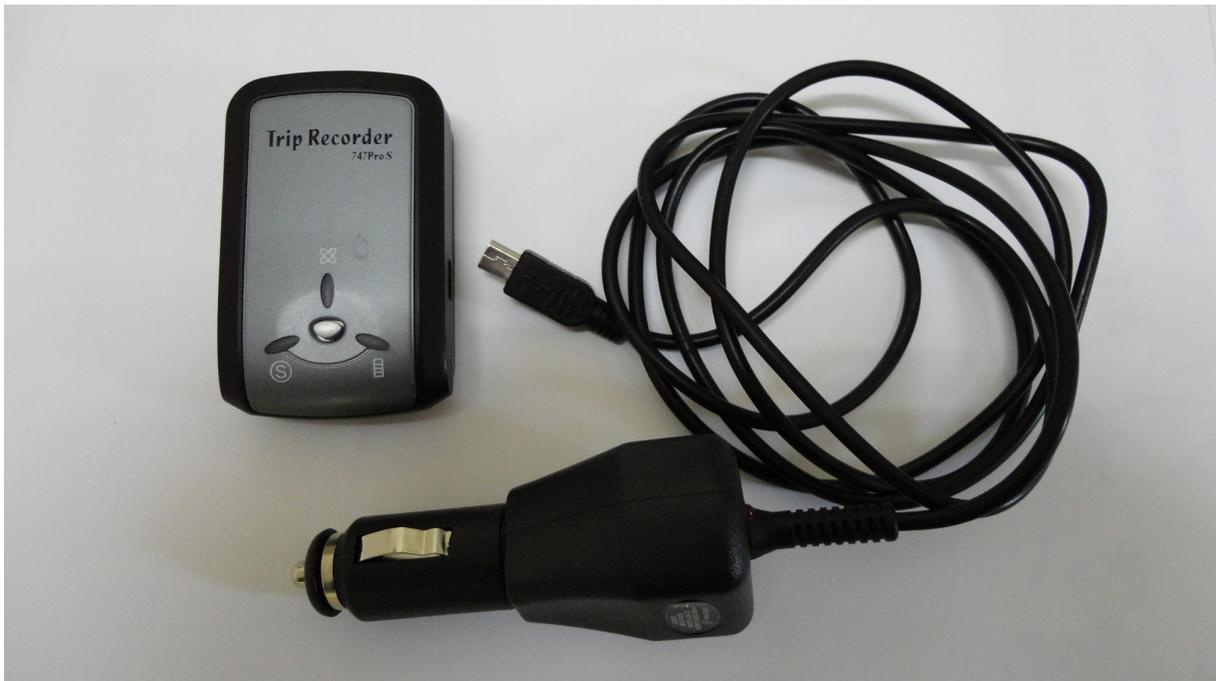
**Figure 1. Digital photograph of the 747ProS GPS Trip Recorder shown with the car charger.**
