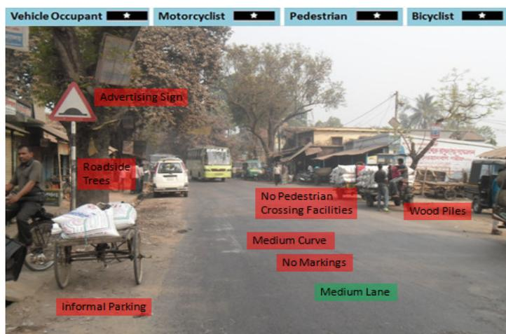
**Figure 8: A 1-star rated section at Prembag, Jessore with associated features**
