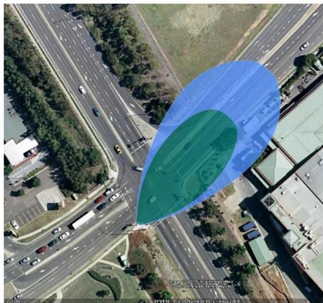
An additional rear facing secondary radar is added to the system if there are requirements for vehicle length determination, vehicle classification and as a recorded speed enforcement crosscheck. The secondary radar is rear facing and installed within the camera enclosure. All radar data for the detected vehicle is saved within the incident and can be analysed by authorised persons at a later time.
