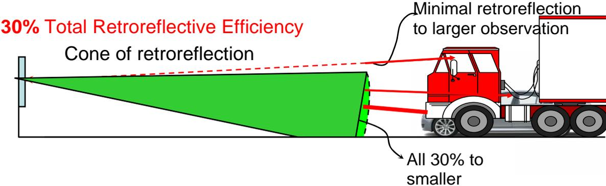
Figure 8A – Light return efficiency of Class 1 sheeting, 3M™ High Intensity Prismatic™ Sheeting
