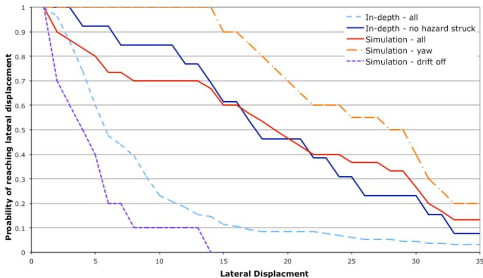
A summary of the average results of the simulations of road departures is shown in Table 2. The difference between the drift off type departures and the departures that involve yawing is once again demonstrated. Of note is the high average impact speed after traversing nine metres of clear zone experienced by the vehicles that were out of control (single and double yaw).
