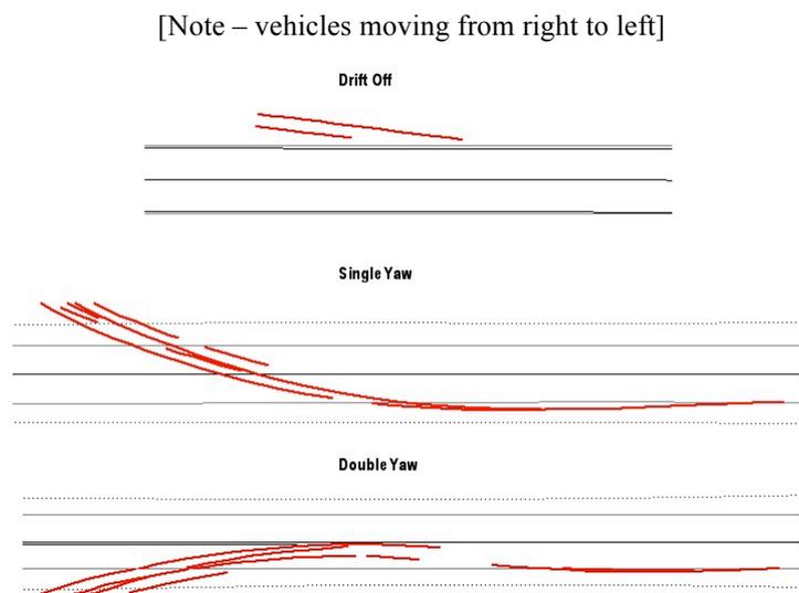
The critical speed method [5,6] was used to calculate the departure speed for all cases involving yawing for which sufficient yaw marks had been recorded on the site diagram. Of the sample of 132 crashes, 71 had sufficient tyre marks to calculate the departure speed.
