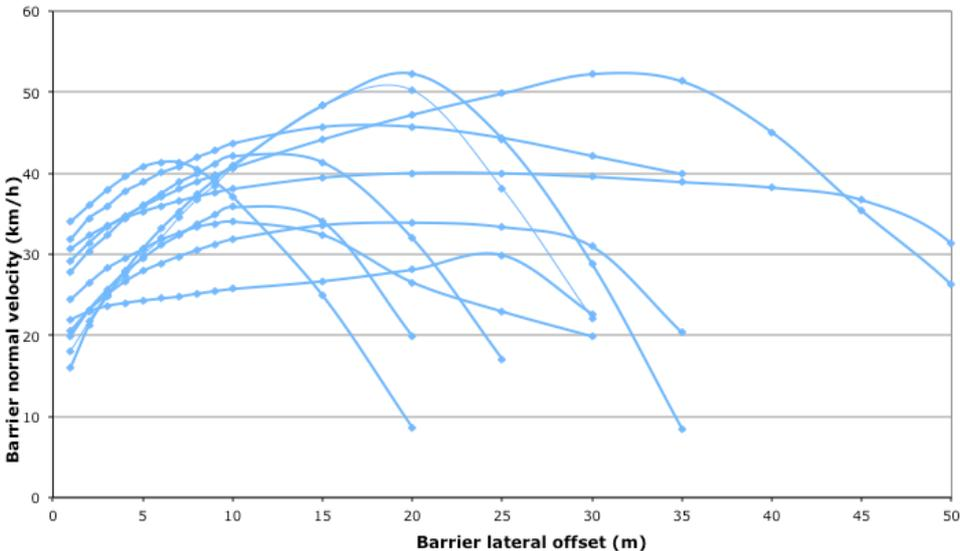
Figure 11 shows the barrier normal velocity relative to the lateral offset of the barrier for loss of control road departures (single yaw and double yaw) using the emergency braking driver scenario. While the plots exhibit the same basic shape as shown in Figure 10 the peak generally occurs at a much smaller lateral offset. The location of the peak is also more uniform than in the results shown in Figure 10. This is because
