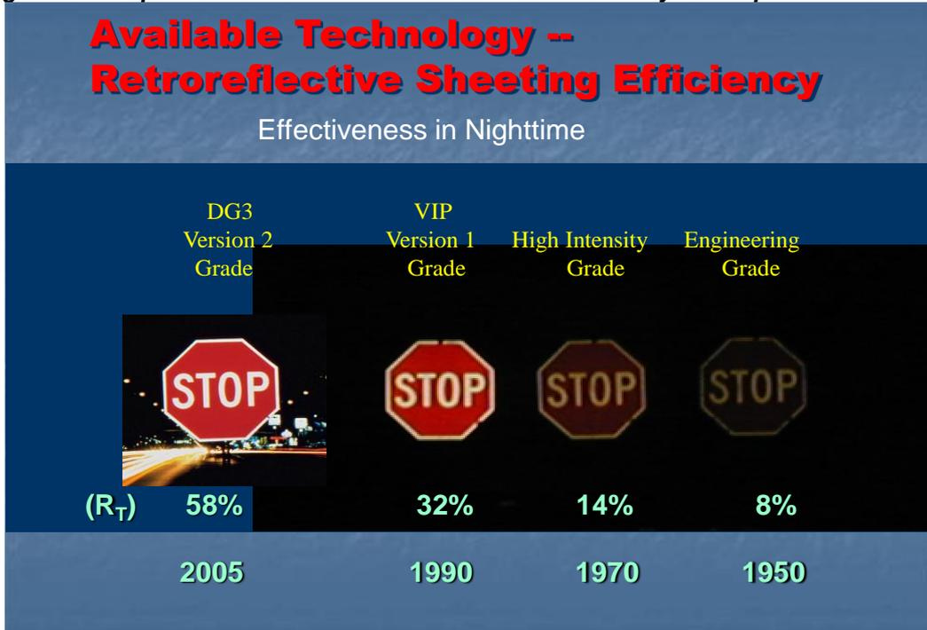
The big advantages in this Full Cube technology is that it provides greater luminance to large vehicles such as trucks that have a large observation angles. It also provides all vehicles greater light reflectivity from disadvantaged sign positions such as signage on the right hand side of the road, overhead gantry positions and winding roads where vehicles headlights do not focus as much light on the sign. (Holderness, 2011)
