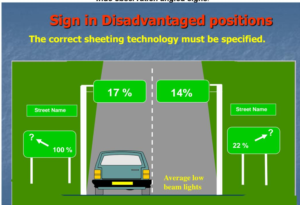
There is also an advantage in the brightness to cater for older drivers and the current move toward the new VOA headlights in new cars which accurately limits the beam angle of headlights. By providing more light to the driver of all vehicle types and improving the sign legibility for disadvantaged signs, 3M's DG3 sheeting is seen as a breakthrough in improving the ability of drivers to read road signage and providing better road safety outcomes.
