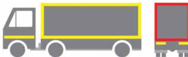
**Figure 9 - Side outline visibility markings can reduce side on collisions by up to 37%.
