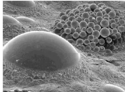
**Figure 5– Magnified image of glassbead and 3M elements**
