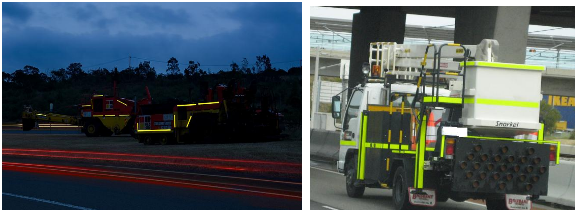
Figure 3 - Roadside vehicles marked up with fluorescent retroreflective materials to increase day and night time visibility
