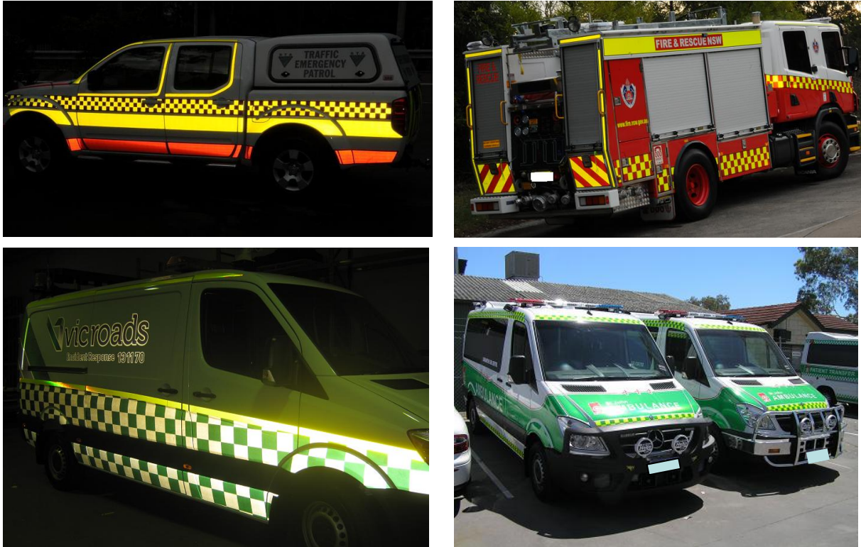
Figure 4- Emergency vehicles marked up with retroreflective and fluorescent retroreflective materials
