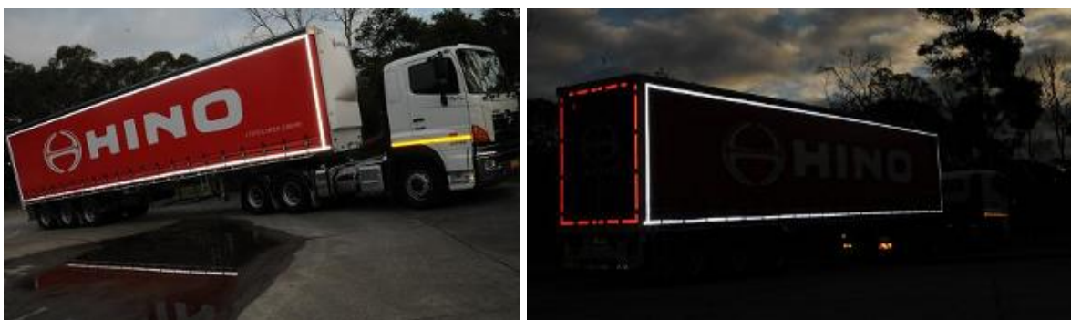
Figure 8 – Trucks marked up according to UN48 / ECE104
