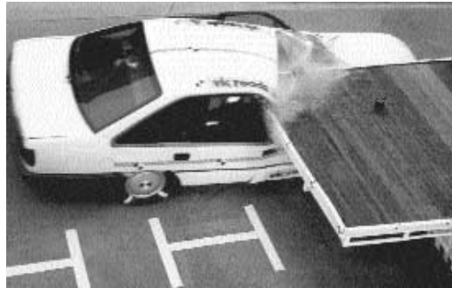
50km/h Offset crash, no rear underrun barrier, 10t rigid truck
