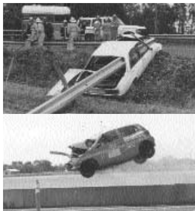
Figure 3: Dangerous roadside barriers. Top: end terminal spearing. Bottom: impacting concrete barrier at large angles is hazardous.
