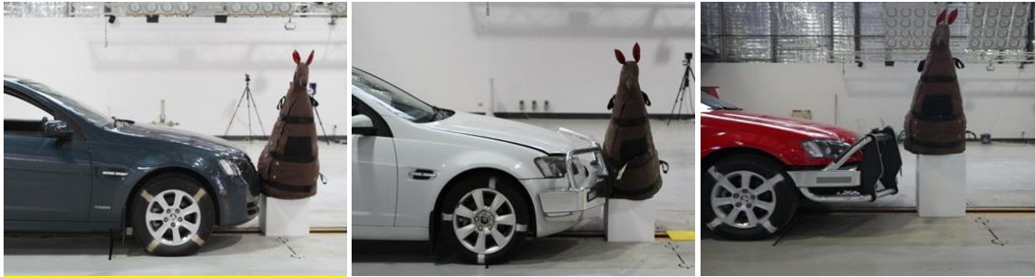
Figure 2.1 Sedan with (L-R): no bull bar, low dummy; urban bull bar, low dummy; rural bull bar, high dummy
