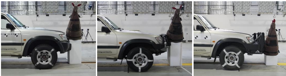
Figure 2.2 4WD with (L-R): no bull bar, high dummy; urban bull bar, high dummy; rural bull bar, low dummy
