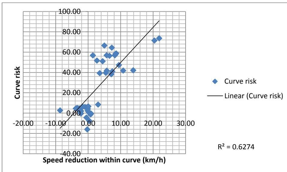
**Figure 3. Mean speed reduction by curve risk**
