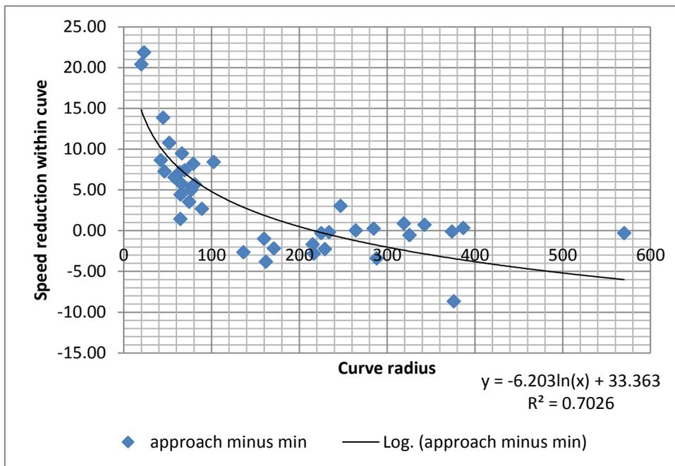
**Figure 2. Mean speed reduction by curve radius**
