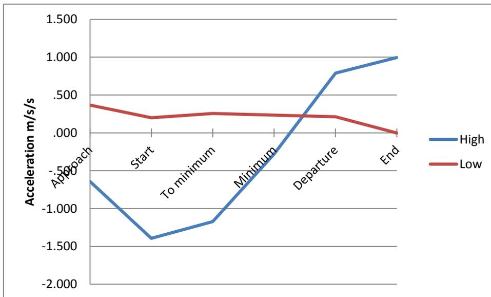
**Figure 6. Mean acceleration/deceleration through curves of different risk**
