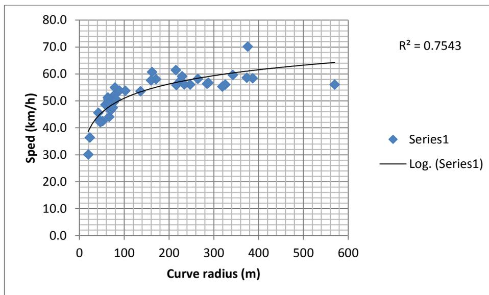
*Figure 1. Mean speed by curve radius*
