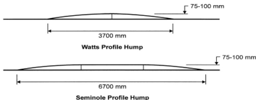
*Figure 1. Watts and Seminole profile road humps*
