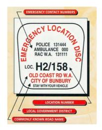
A total number of 150 discs have been installed on markers by members of South West Rotary Clubs. The discs are placed both sides of the Old Coast Road carriageway and are off set providing one disk every 500 metres (see diagram below). Where the markers have been placed is within mobile phone range so that mobile phones can be used to call emergency services in the case of a road trauma incident or other emergency situation.
