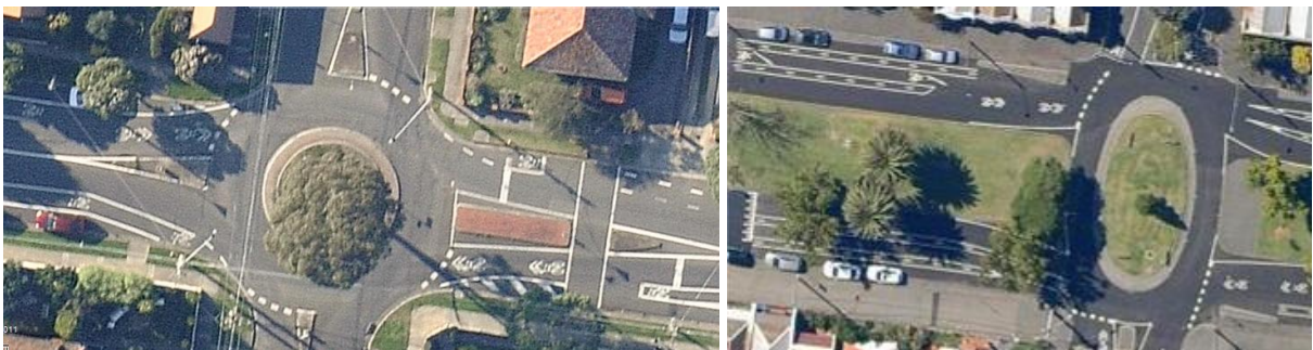
Figure 7: Rural City of Mildura (Vic) –San Mateo Ave & 12th St Design includes: bicycle logos in middle of lanes (entry and circulating); bicycle symbols with merge arrows; Riley Kerb mountable geometry tightening (to allow B-doubles) and approach slowing; BIKE MERGE AHEAD pavement warnings; & “bicycles / merge right” signage. Installed 2012.
