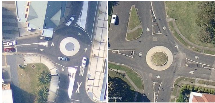
Figure 6: City of Darebin (Vic) –Raglan St, Preston & City of Yarra (Vic) Pigdon St, Carlton Designs include sharrows in the middle of lanes and bicycle symbols with merge arrows. Installed July 2011 & Feb 2012.
